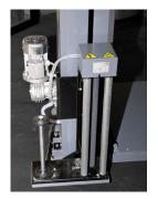
**Electromagnetic film tension** with easy film threading
