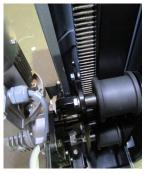
Rack & Pinion carriage drive system for added reliability
