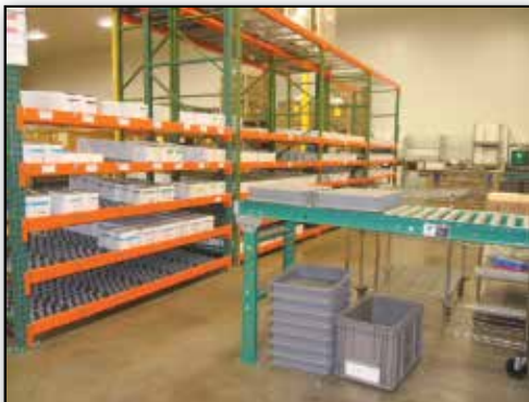
Span track rollers are ideal for hand picking applications at ground levels.
