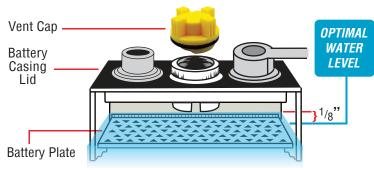
Optimal Water Level is about one eighths inch (1/8") above the Battery Plate - water should just barely cover battery plates under the battery casing lid.
