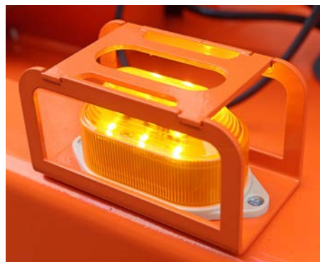
Dual flashing beacons alert pedestrians during operation.
